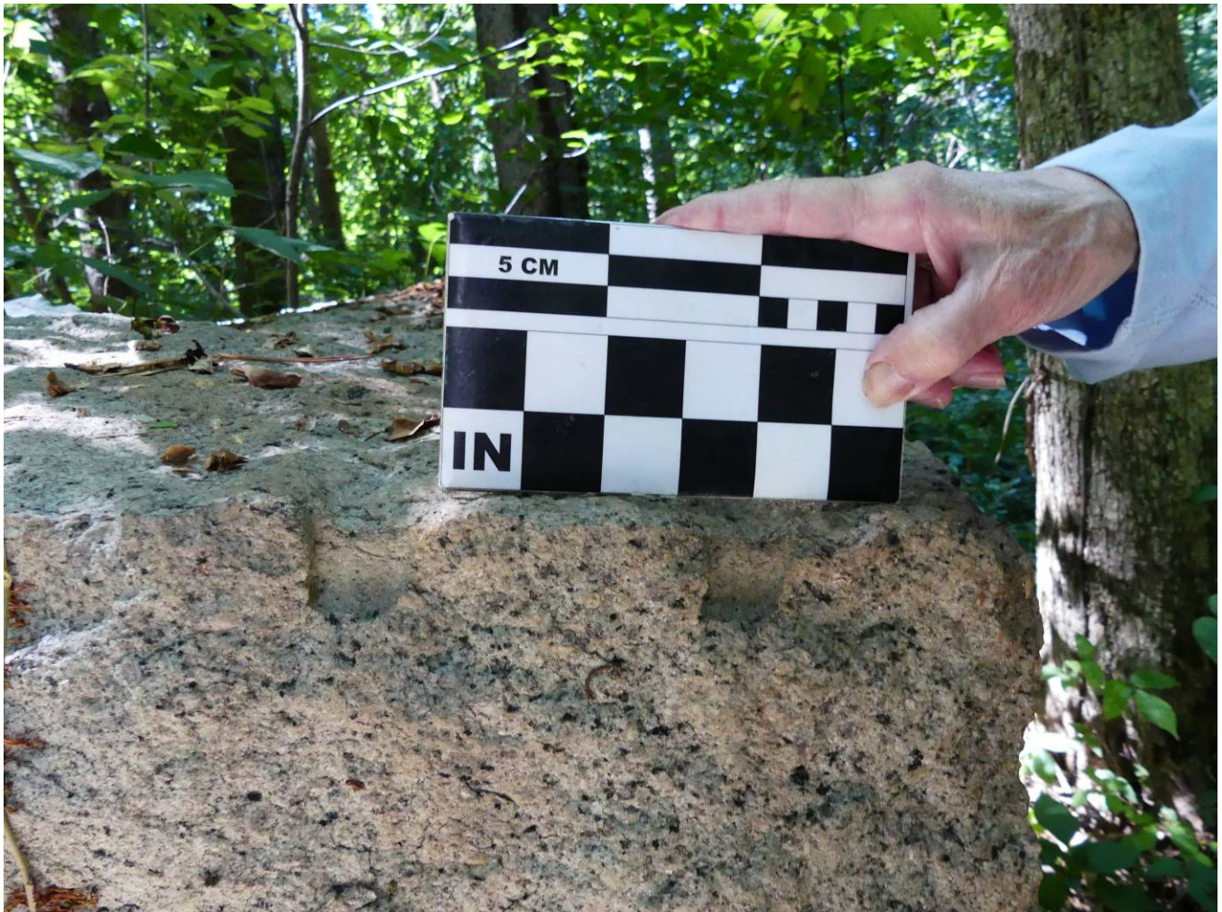
Figure 22 – Tools marks from an 1868 rock hammer. These are small shallow flat square holes that are much smaller than the larger trapezoid shaped flat wedge holes that were hand chiseled.
