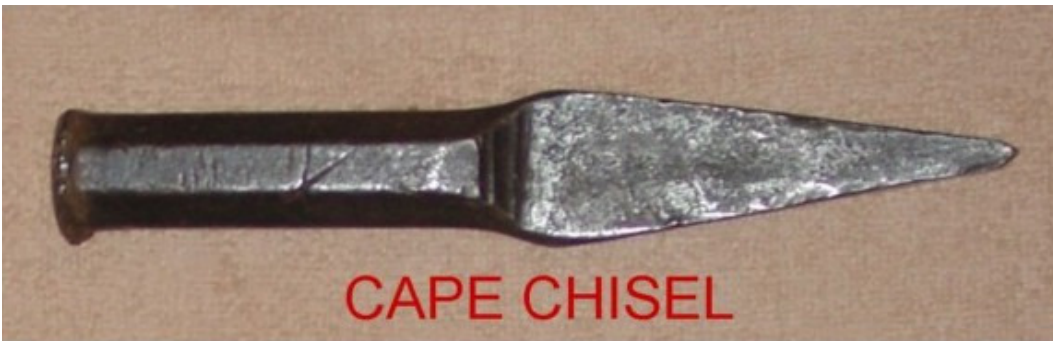
Figure 53 – Cape Chisel used to make flat wedge holes.
