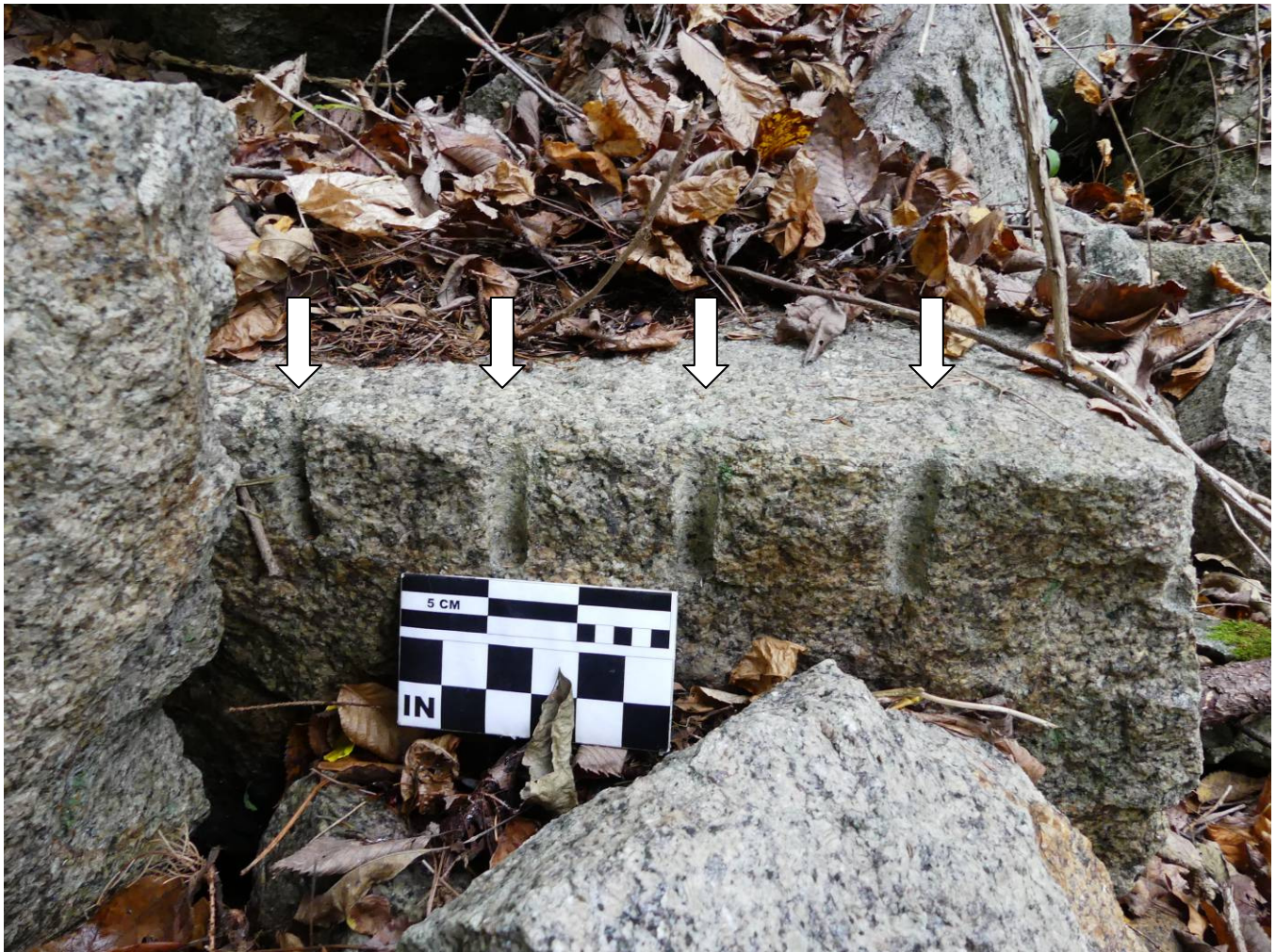
Figure 20 – Plug and feather drill marks.
