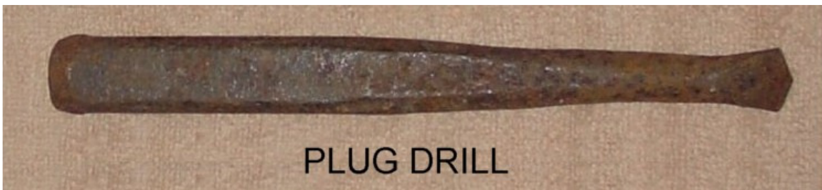
Figure 54 – Plug drill used to make round holes with rounded bottoms.
