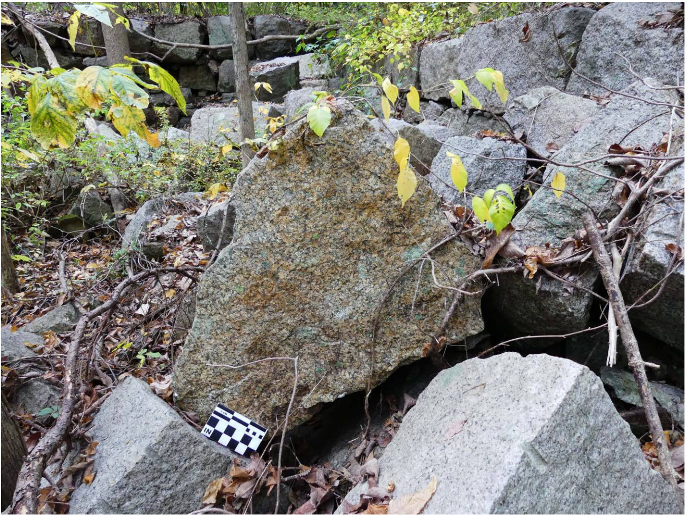
Figure 19 – Quarried stone blocks were located in the north wall and loose on the ground inside the foundation. These blocks were commercially quarried but were grout (a.k.a. waste) quality. Some had odd shape like the one shown in this photo.
